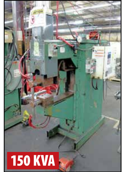
150 KVA METHODS MPT1S-30-50 SPOT WELDER
