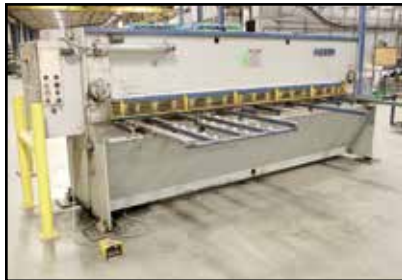
LVD JS 2510 10' X 1/4" HYDRAULIC SHEAR
